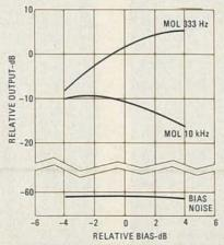
FIG. 1—THE BIAS LEVEL that provides the highest output with acceptably low distortion for a 333-kHz tone is quite different than the bias level required by a 10-kHz tone.
