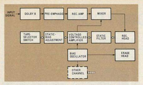
FIG. 5—BLOCK DIAGRAM of the Dolby HX Professional system. Unlike Dolby HX, this system measures the sum of the audio signal, including any preprocessing, and the bias at the record head.
