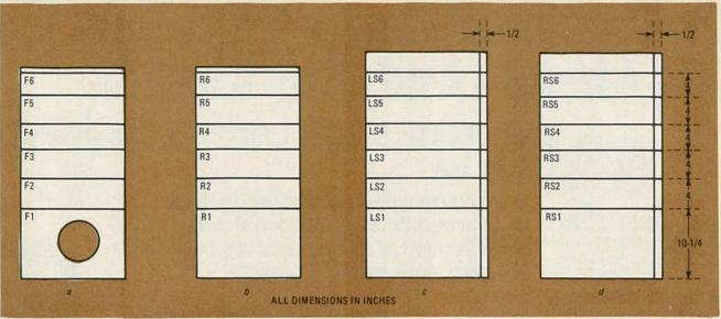
FIG. 8—PARTITION MOUNTING STRIPS for the front are shown in (a), rear are shown in (b), left side are shown in (c) and right side are shown in (d).
