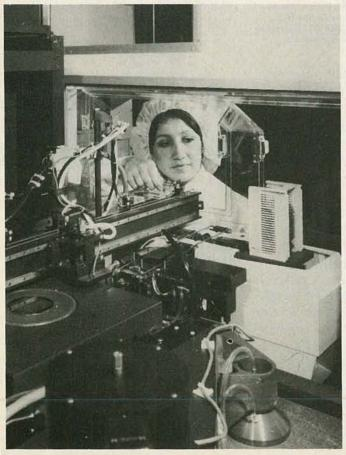
PHOTO-LITHOGRAPHY MACHINE that will be used to etch VHSIC circuits on chips the size of a thumbtack. Hughes and five other firms are in the program conducted by the Defense Department to develop the high-speed superchips. The machine is being operated by Hughes technician Margaret Sanchez.
