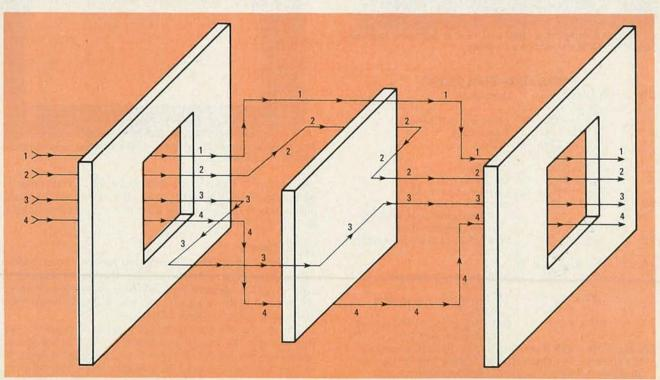
FIG. 2—SPEAKER BACK-WAVE is alternately combined and separated as it passes through and around SAFE enclosure's baffles.
