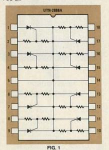
Characteristics of any individual SCR (maximum limits are given unless otherwise specified) are: Forward blocking-current, 50 µA; gate-to-anode leakage, 250 µA; forward on-voltage, 1.2 volts at +25°C and 1.15 volts at +55°C; gate trigger-voltage, 2.5 volts; gate trigger-current, 300 µA; gate OFFcurrent, 10 µA; holding current, 10 mA at 0°C and 5.0 mA at +55°C, and anode OFF-voltage, 400 mV minimum.
