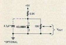
FIG. 7—A 1.2-VOLT temperature-compensated voltage reference, the Intersil ICL8079 used in this circuit is well suited to high-speed A/D and D/A converter projects.
