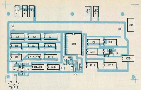
FIG. 4—SOCKET SO1 is a 24-pin zero-insertion-force socket used to hold the 2716 EPROM. Zeroinsertion-force sockets allow IC's to be inserted and removed many times without causing wear or damage to either the socket or the IC.
