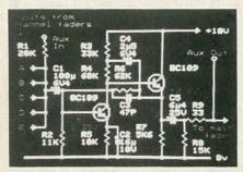
FIG. 15—A DYNAMICALLY REDEFINABLE character set (DRCS) makes the presentation of pictures such as this schematic relatively easy.
