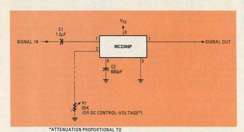
FIG. 1—THIS SIMPLE ATTENUATOR CIRCUIT allows you to control the volume of a receiver hidden in the trunk of your car with a dash-mounted potentiometer.
