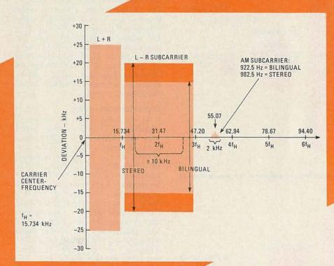
FIG. 1—ORIGINAL EIAJ SYSTEM uses a subcarrier with a deviation of ±10 kHz to transmit the L-R or second-channel audio information. Maximum frequency-response is 12 kHz.
