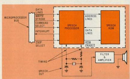
FIG. 1—A TYPICAL IC SPEECH-SYNTHESIZER uses a ROM containing speech data, circuitry to process the data and turn it into analog form, and an amplifier and speaker.
