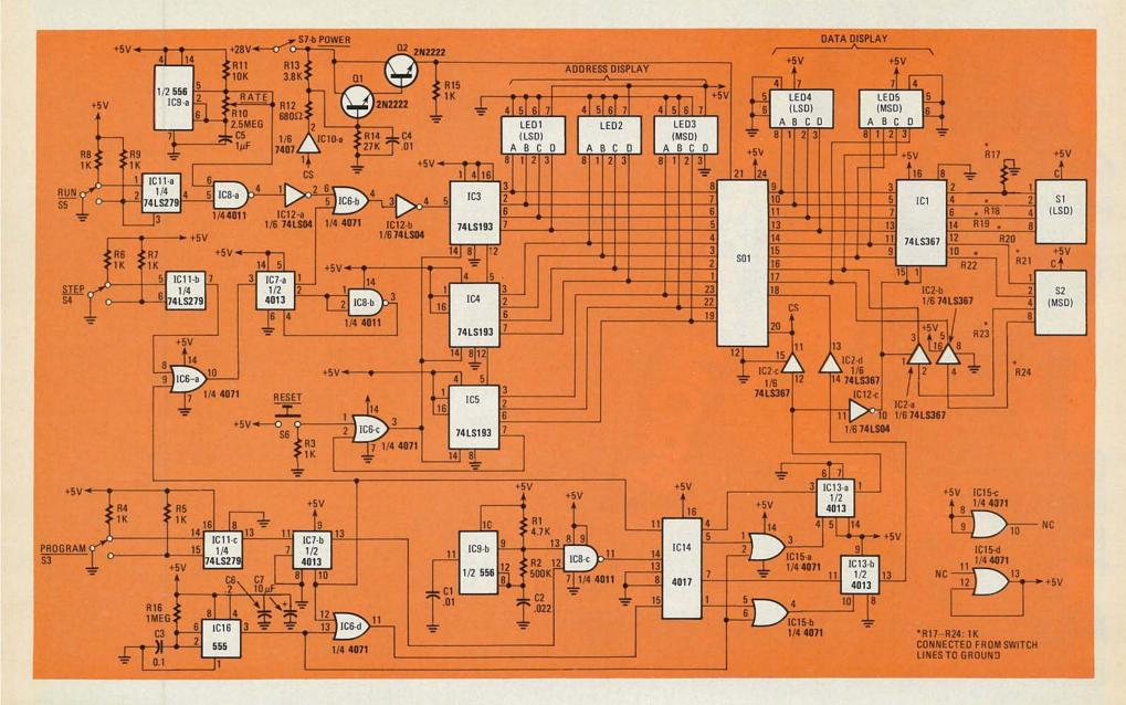
FIG. 1—WHILE ONLY R17 IS SHOWN, resistors R17-R24 are connected from the eight output-lines of S1 and S2 to ground.
