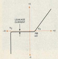
FIG. 2—WHEN THE REVERSE BIAS exceeds V<sub>Z</sub> the negative current through the Zener increases rapidly.
