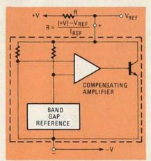
FIG. 6—THIS TWO-TERMINAL REGULATOR from Ferranti Electric can be used just like a Zener diode. It has a stability as great as 10 ppm per 1000 hours of operation.
