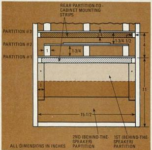
FIG. 5—NON-PERSPECTIVE VIEW from front of enclosure. Note construction of partition 1/partition 2 assembly.
