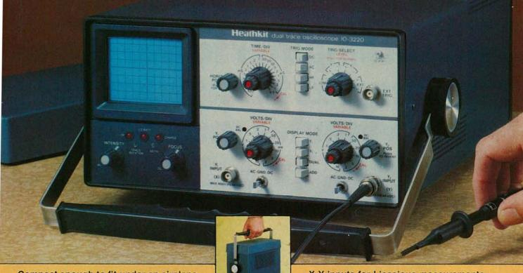
Compact enough to fit under an airplane seat, the Heathkit IO-3220 represents outstanding value in its class. Weighing only 16 pounds, the IO-3220 is designed for field service troubleshooters who need a light, portable battery-operated scope for use where AC power is not available.
