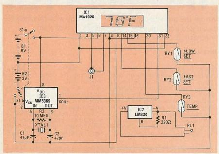
FIG. 3-FOR PORTABLE OPERATION, build this version of the clock/thermometer project. The oscillator circuit draws just 1.5 milliamperes.
