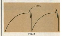
You'll find one waveform at some points that you'll never see in tube-type circuits—a perfect sawtooth. With tubes, the signal on the oscillator grid (Fig. 2) shows the familiar rising curve with a spike at the top. Solid-state oscillators, on the other hand, show a
