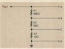
FIG. 11-A RESISTOR NETWORK can be used to get a multiple-output voltage reference. The voltage at each tap is 10 times higher than the voltage at the tap below it.
