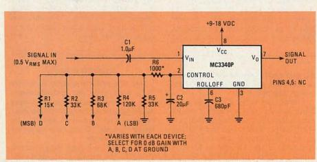
FIG. 2—SCHEMATIC DIAGRAM of a digitally-controlled attenuator circuit. Lines A, B, C, and D, can be driven by the simple circuit shown in Fig. 4.
