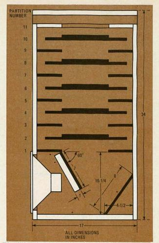
FIG. 6-SIMPLIFIED CUTAWAY VIEW of enclosure showing mounting details of first and second behind-the-speaker partitions.
