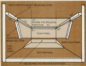
FIG. 4—EXAGGERATED PERSPECTIVE VIEW of first chamber. Note mountings of first and second behind-the-speaker partitions.
