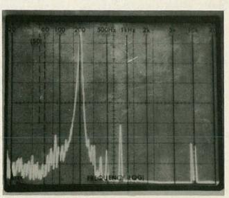
FIG. 4—MUTUAL BIASING is demonstrated here. Two low-level, higher-frequency (9 and 10 kHz) tones were mixed with the 300-Hz tone.
