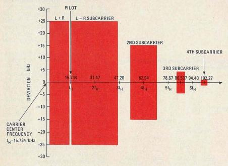
FIG. 4—ZENITH RADIO CORPORATION'S system uses the horizontal line-frequency, 15.734 kHz, for the pilot tone.
