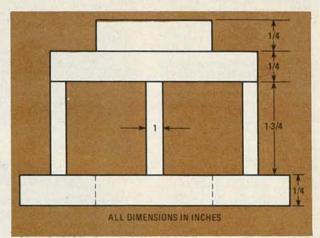
FIG. 11—SIDE VIEW of even-numbered partition mounted atop odd-numbered partition using partition mounting strips. Each strip is located as shown in Fig. 10 and measures 1  $\times$  1  $\times$  1% inches.
