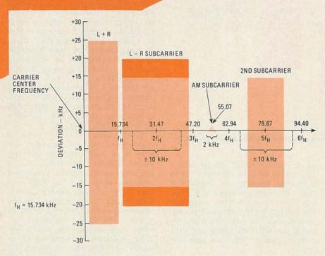
FIG. 2—U.S. VERSION of the EIAJ system extends frequency-response of the subcarrier to 15 kHz. In addition, a second subcarrier, with an 8-kHz bandwidth, is provided for.
