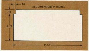
FIG. 7—FIRST BEHIND-THE-SPEAKER PARTITION has cutouts to accommodate mounting strips.
