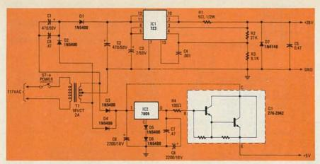
FIG. 2—POWER SUPPLY provides both the 5-volts needed for the logic circuitry and the 25.5-volts used to program the EPROM.
