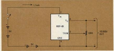
FIG. 10—A SIMPLE POTENTIOMETER is used to trim the output of the PMI REF-01 voltage reference to exactly 10.00 volts.
